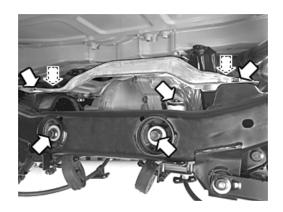
housing. Leave the screws in place by a few threads.
