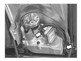
Install the propeller shaft on the final drive. Install the member for the center bearing. See: Propeller shaft, replacing.
