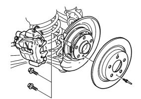
removed from the wheel spindle.
