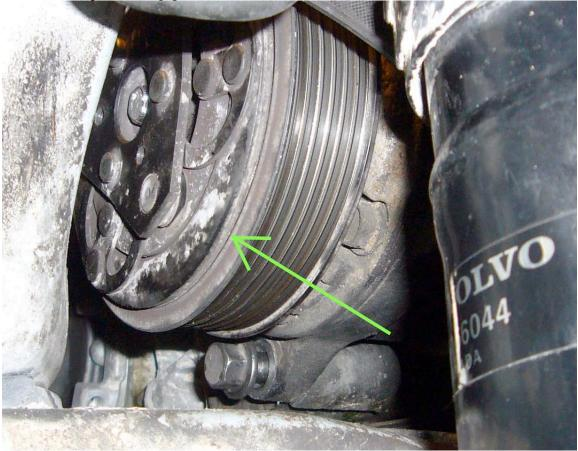
To remove the clutch plate, you'll need a little bit of space to work. Remove the serpentine belt and remove mounting bolts for the compressor. There are 4 bolts that hold the compressor in. They are all located on the side of the compressor that is towards the back of the car. There are 2 bolts on the pulley side of the compressor and 2 on the hose
