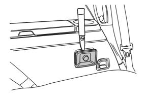
Cut six  $8 \times 20$  mm pieces of felt material with P/N 116 1691. Apply two pieces of felt to the top of each lug.
