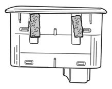
Apply a piece of felt to the bottom of each lug.
