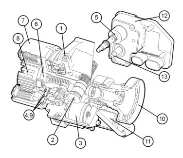
The hydraulic section consists of 1-5, the mechanical consists of 6-10 and the electronic section consists of 11-13:
